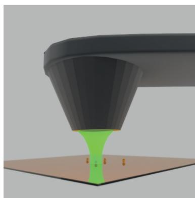
atomic force microscope cantilever. The micromirror faces a planar dielectric mirror to form a plane-concave microcavity
