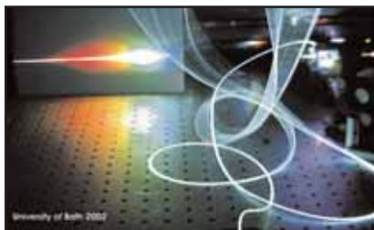
Figure 4: White-light supercontinuum (10,000 times brighter than the sun) generated in PCF with zero dispersion at  $800 \text{ nm}$ , pumped by  $150 \text{ fs}$  Ti:sapphire pulses of energy  $1\text{-nJ}$ .
