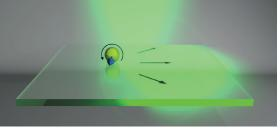
and the transverse field components in tightly focused radially polarized light, the dipole moment can be controlled via careful positioning of the nanoantenna relative to the axis of the excitation beam incident normal to the substrate. The emission direction then depends on the azimuthal position of the particle. As an application, we used this concept for selective directional coupling into a dielectric waveguide (see figure).
