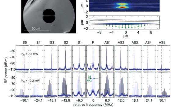
tors, where frequency combs are generated via the electronic Kerr nonlinearity, the underlying mechanism in our case is stimulated Raman-like scattering (SRLS), mediated through optical gradient forces and initiated by thermally excited phonons. This is the first demonstration of noise-seeded, optomechanical SRLS – a
